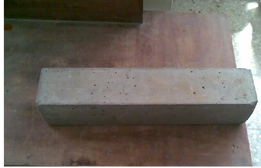
Figure (3.21): Prism flexural test specimens (100*100*500mm)
