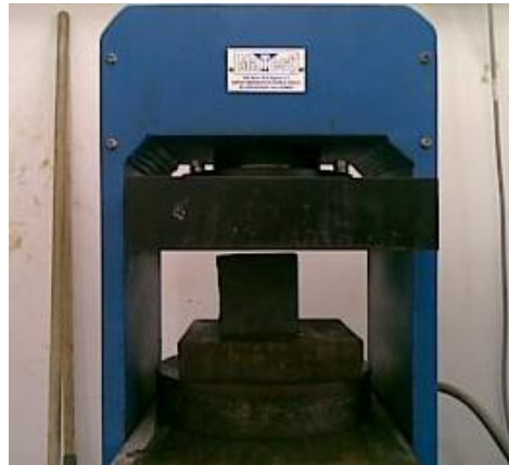
Figure (3.16): Compressive strength test machine
