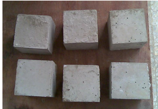
Figure (3.15): Compression test specimens (100x100x100mm)
