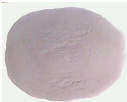
Figure (3.10): The silica fume used in mixtures preparation.
