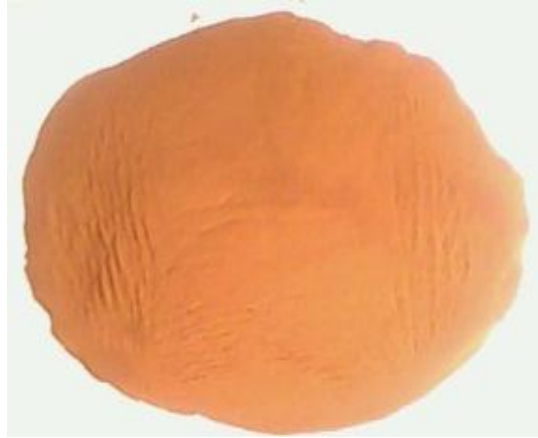
Figure (3.9): The chemical admixture (Superplasticizer) used in mixture preparation.
