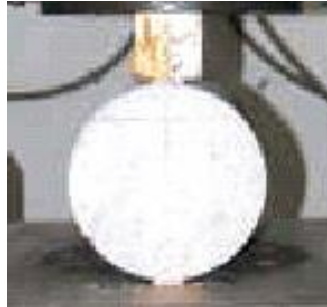
Figure (3.17): Split cylinder test setup for cylinder 150 x 300mm
